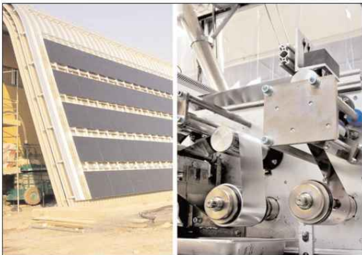
Shell Solar CIGS PV installation in Wales, UK (left) and roll-printing at Nanosolar (right). Credit: NREL.
